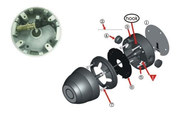
Here is the location for drainage, please follow the arrows downward direction to install
